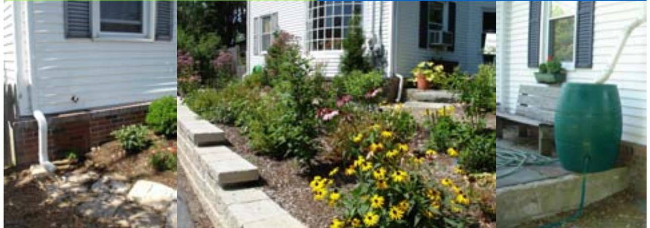
The rain garden captures roof runoff from three down spouts, and a rain barrel captures the fourth. We use water from the rain barrel to irrigate when necessary.
